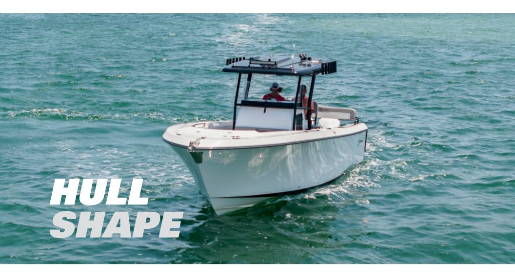
Engineered for navigating rough seas with safety, comfort, and not getting wet. With its deep-V hull design featuring inward lines, it ensures optimal performance for slicing through waves, preventing water spray from reaching passengers. This design delivers an excellent balance of speed and fuel efficiency during voyages.
